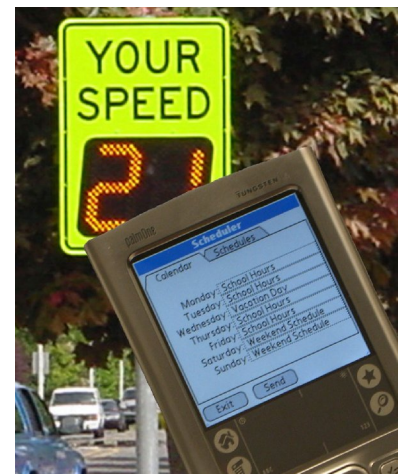
The SpeedCheck Remote Scheduler allows fast wireless setting of display features.
